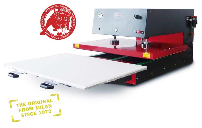
LTS 609 is an automatic press with a pneumatic function.
